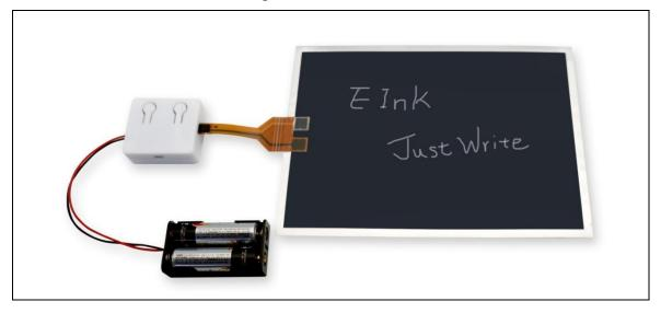
• Turn the battery power and driving board switch to "on". Red light can be seen on the shell when power is on.
